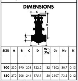
Cv = Flow Coefficient US Gal/min. to give 1 psi pressure drop. Kv = Flow Coefficient L/s to give 1 kPa pressure drop. K = Dimension less resistance Coefficient. Dimensions in mm. Weights in Kg.
